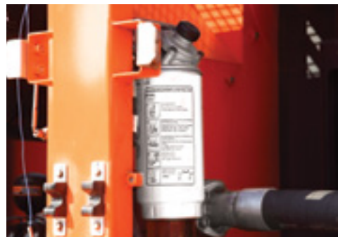
Fuel pre-filter with water separator High efficiency fuel filtration is attained by the use of multiple filters. These include a fuel prefilter fitted with a water separator that removes moisture, dirt and debris from the fuel. A fuel drain valve has been installed to facilitate maintenance.
