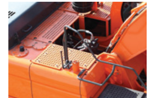
Cat walk (platform) as standard on DX420LCA Larger anti-slip surface on the upper structure for more safety.
