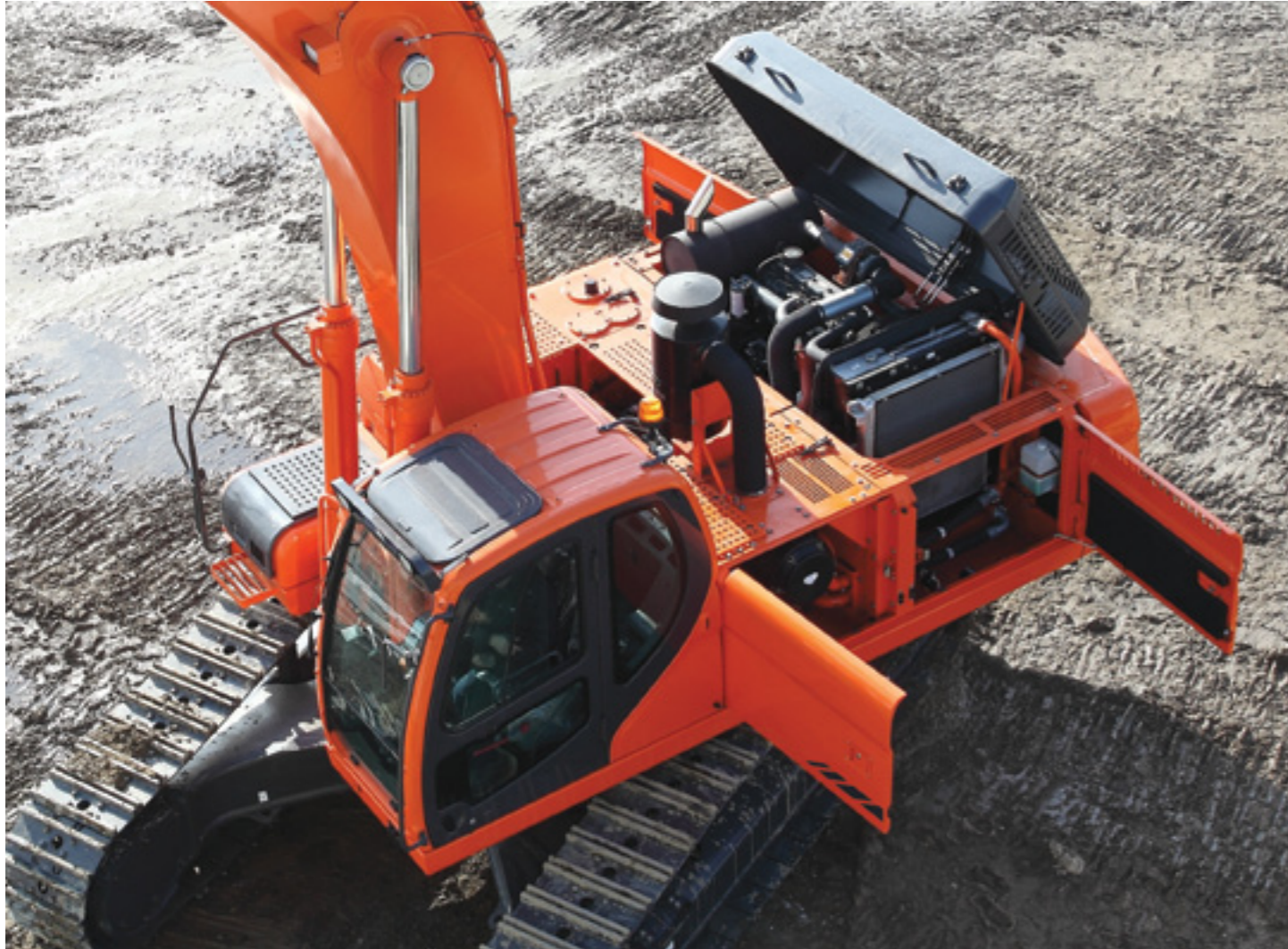
Accessible parts Access to the various radiators is very easy, making cleaning simpler. Engine parts can be easily reached via the top and side panels.
